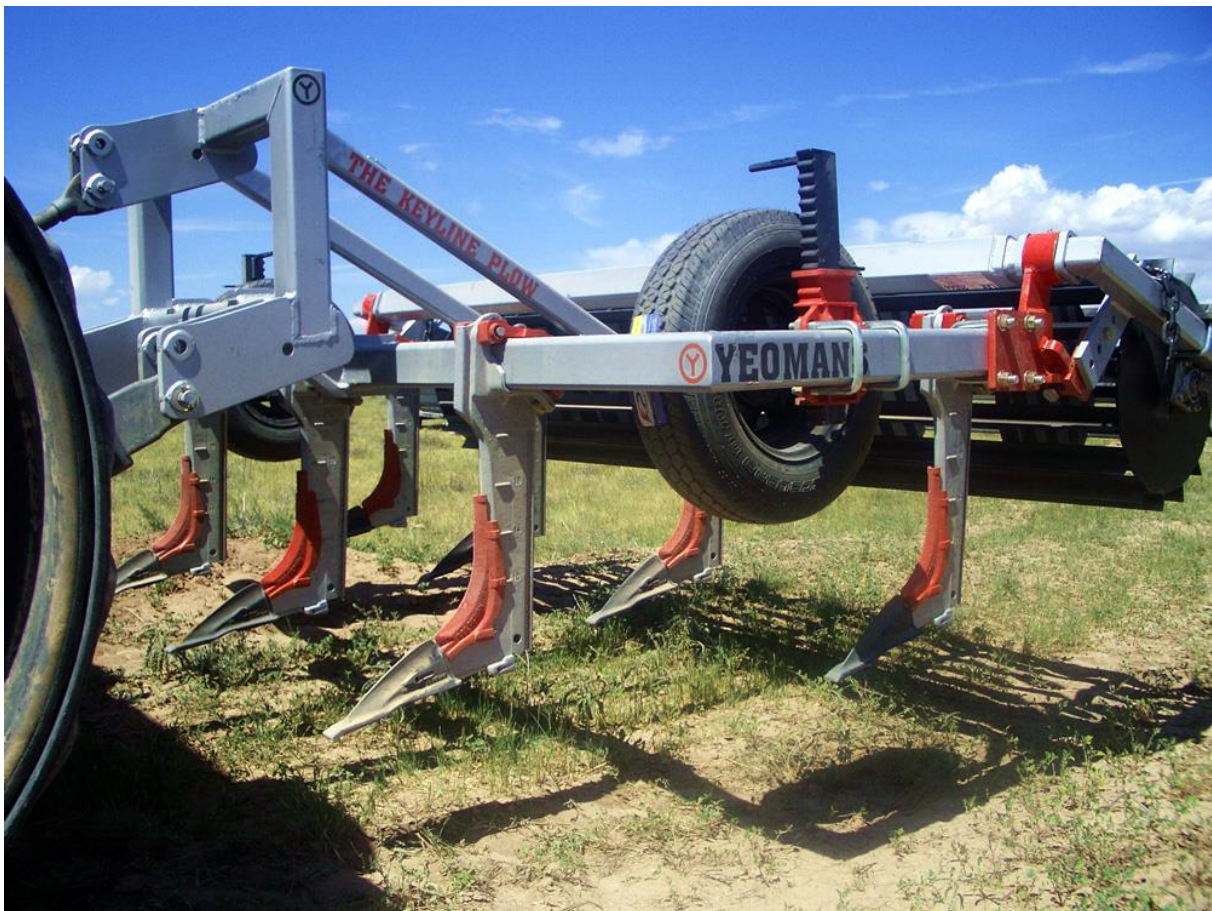
Figure 2: Yeomans Keyline plow (Hokonui.com, 2014).
