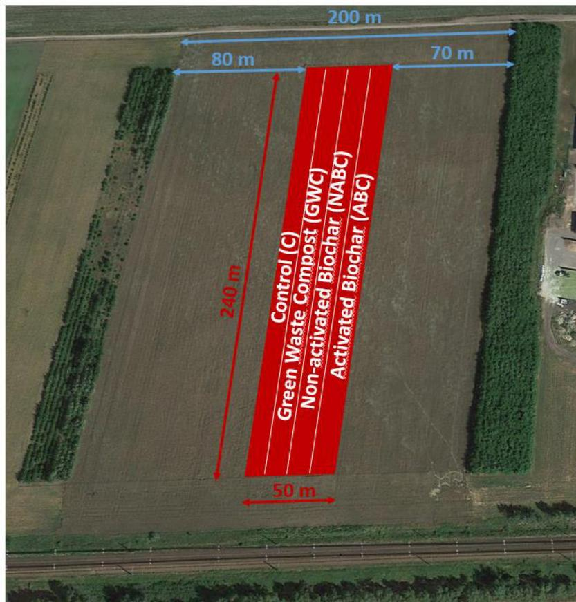
Figure 2: Arrangement of the variations at the experimental site in Peickwitz, Germany
